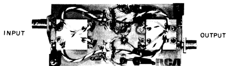
Fig. 6— Physical layout of the 100-watt push-pull amplifier.
